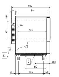
Drain Electrical inlet (power)
